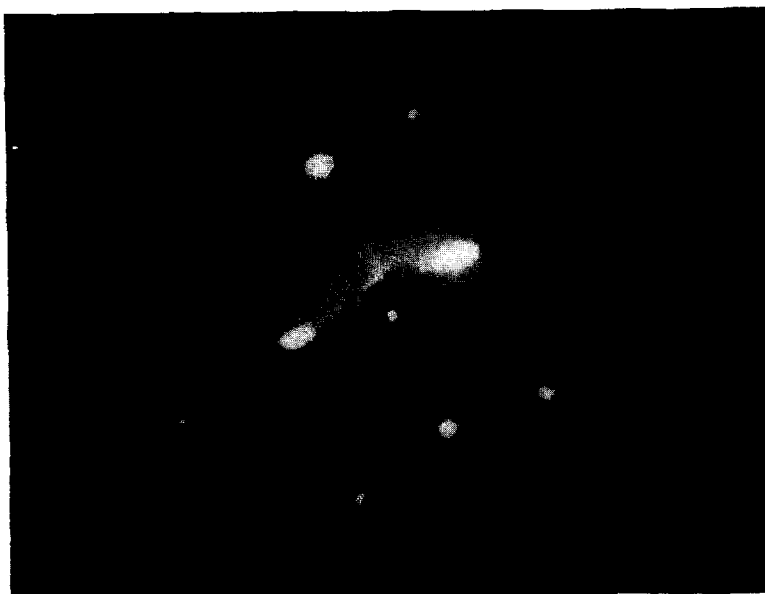
FIG. 2. LEED pattern of a 1 \times 3 structure due to coadsorption of hydrogen and carbon monoxide.
